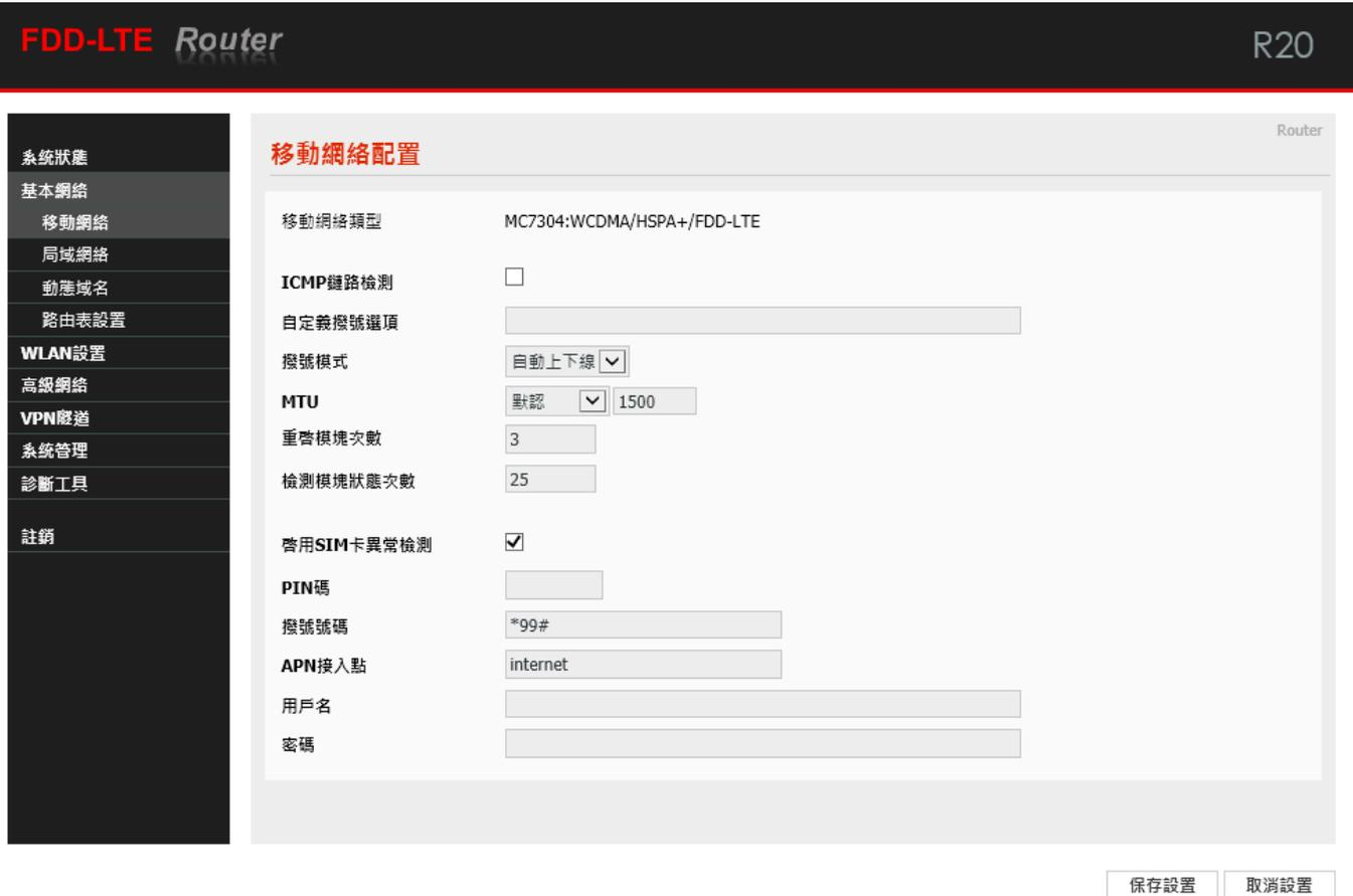
The screenshot shows the '移動網路配置' (Mobile Network Configuration) page of an FDD-LTE Router. The page title is 'FDD-LTE Router' and the model is 'R20'. The left sidebar contains a navigation menu with items like '系統狀態', '基本網路', '移動網路', '局域網路', '動態域名', '路由表設置', 'WLAN設置', '高級網路', 'VPN隧道', '系統管理', '診斷工具', and '註銷'. The main content area is titled '移動網路配置' and includes the following settings:
