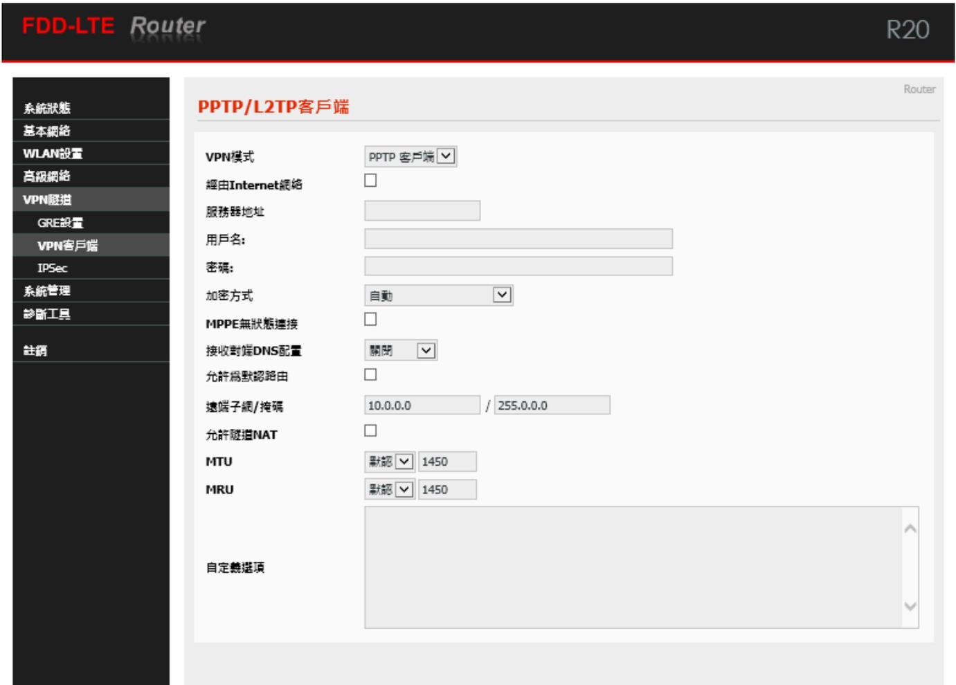
The screenshot shows the configuration page for PPTP/L2TP Client on an FDD-LTE Router. The page title is "PPTP/L2TP客戶端" and the router model is "R20". The left sidebar contains navigation options: 系統狀態, 基本網絡, WLAN設置, 高級網絡, VPN隧道, GRE設置, VPN客戶端 (selected), IPSec, 系統管理, 診斷工具, and 註銷. The main configuration area includes the following fields:
