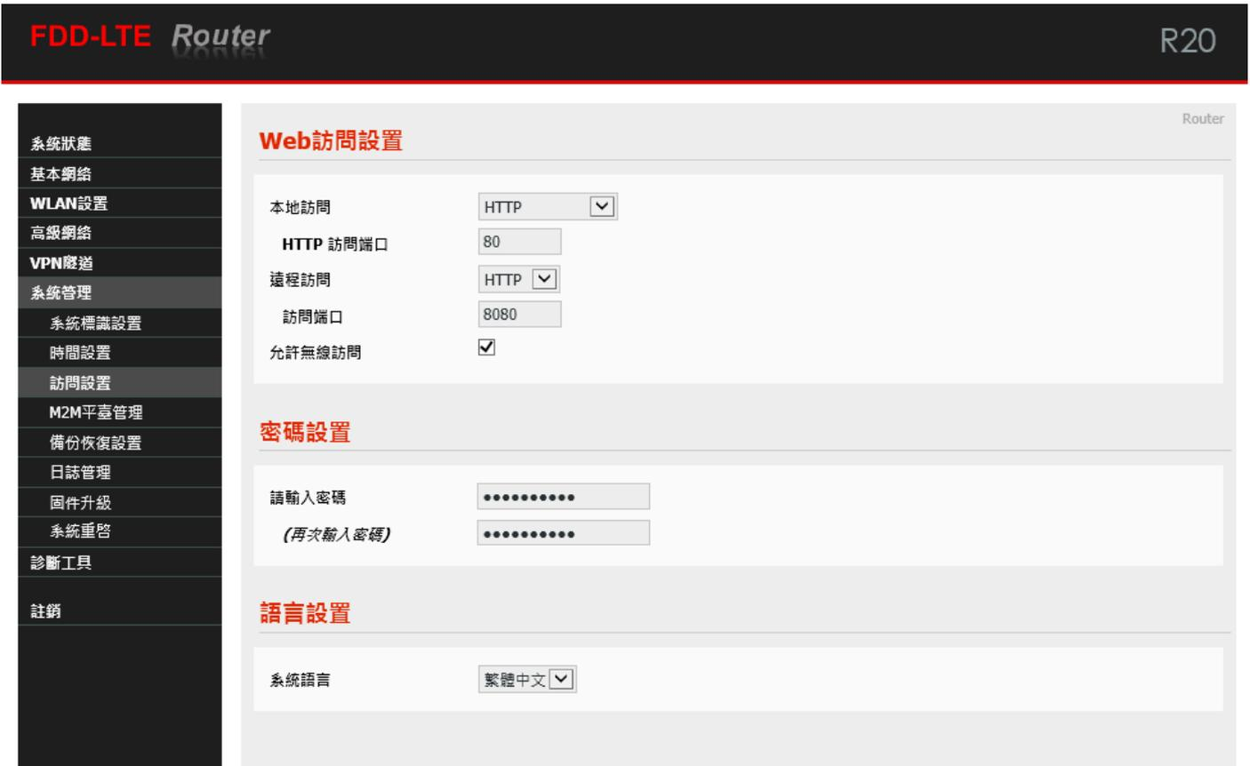
The screenshot shows the web management interface for an FDD-LTE Router R20. On the left is a navigation menu with options like System Status, Basic Network, WLAN, VPN, System Management, and System Language. The main content area is divided into three sections: Web Access, Password, and Language.
