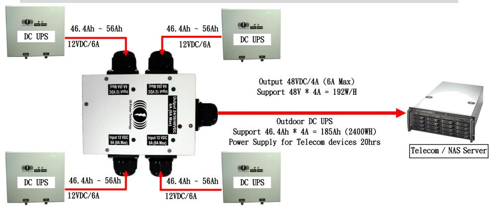
Insert 2 x 12VDC power supply voltage in series, the output voltage automatic step-up 24VDC power supply Insert 3 x 12VDC power supply voltage in series, the output voltage automatic step-up 36VDC power supply Insert 4 x 12VDC power supply voltage in series, the output voltage automatic step-up 48VDC power supply
