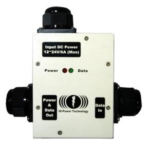
IO-Power DPOE-PSP1248-OB series are an outdoor DC to DC Power over Ethernet (PoE) Converter. To respond to outdoor DC UPS power system, the power source is from online outdoor DC UPS system or general 12~24VDC power adapter and Vehicle 12V/24VDC car cigarette lighter power sources. Complete with DC to DC PoE, supplying power for the device through Ethernet cable (RJ-45). At the same time, it has the Ethernet cable data transmission ports, so it can transmit the data out of the device.
