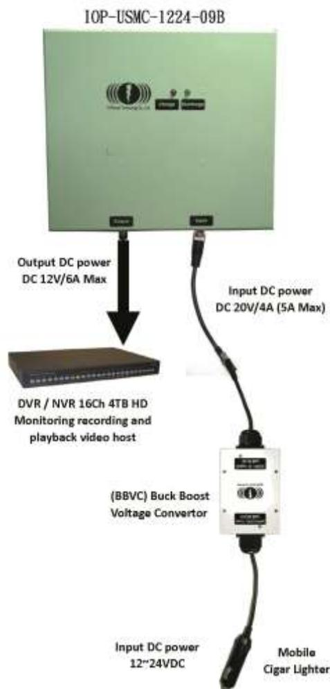
IOP-USMC-12V1224-OA series is specifically designed for large power equipment vehicle load system, through vehicle cigarette lighter-powered uninterruptible operation of the system, such as on-board infrared camera, car video host, DVR/NVR 48 hour record, the range of temporary large discharge current device must be over 48 hours or longer-lasting forms online without interrupting the operation of the power system.
