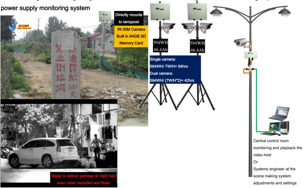
Case 3: "Temporary active video surveillance"- Fireworks spells area / watch Fireworks spells area -- real-time wireless surveillance system of mobile power supply
